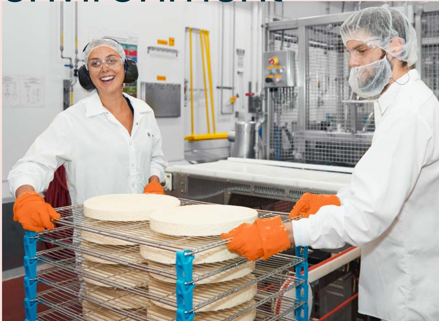
Saint-Hyacinthe plant employees Marie Chainière and Dominic Gadbois removing cheese from moulds prior to ripening.
